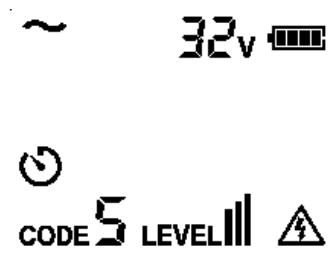
Figure 9.1f AC voltage (&gt;30V) measurement
