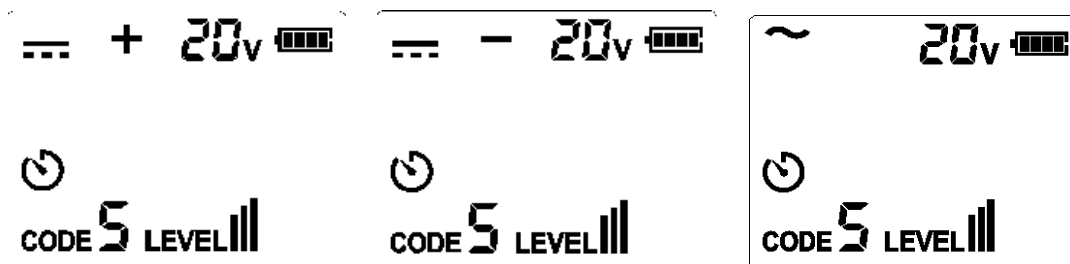
Figure 7.1.2b Voltage below 30V
